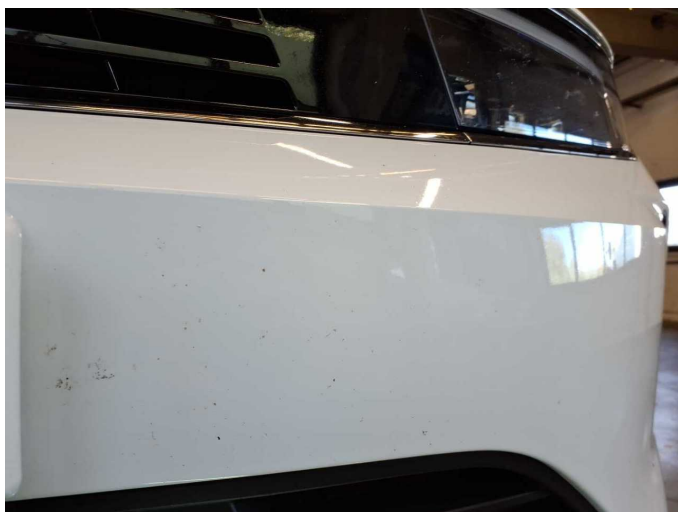
Damage 9: Front bumper: Front bumper - Scratch(es) - Paint
