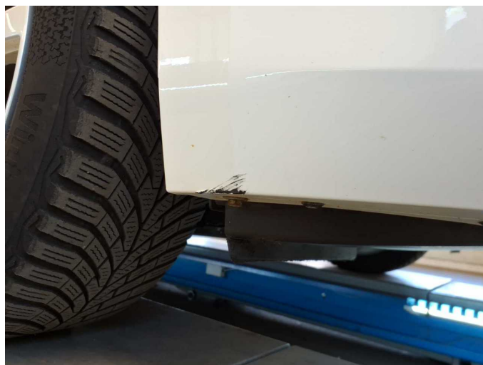
Damage 9: Front bumper: Front bumper - Scratch(es) - Paint
