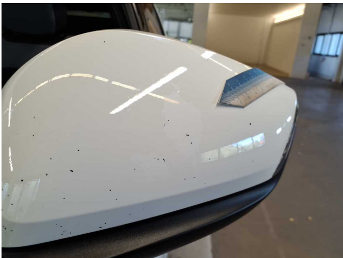
Damage 2: Wing mirror - left side: Cap (Klarlackmangel) - Paint defect - Smart repair
