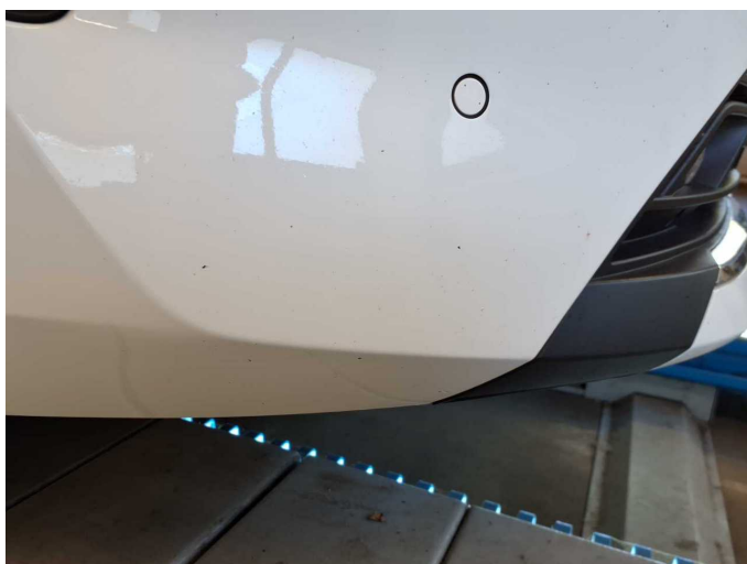
Damage 9: Front bumper: Front bumper - Scratch(es) - Paint
