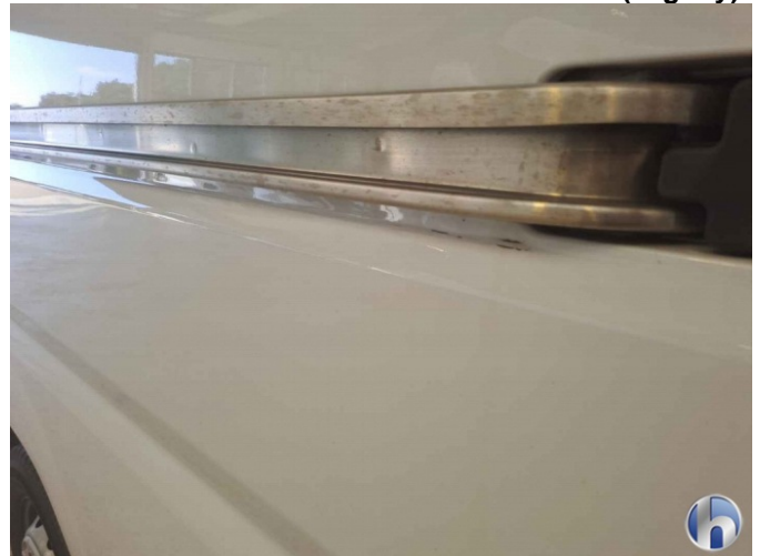
5. Sidewall - Rear - right Deformed (slightly)
