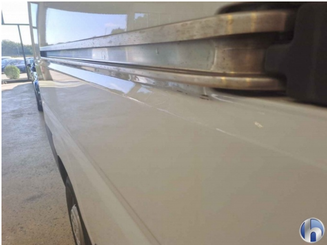
5. Sidewall - Rear - right Deformed (slightly)
