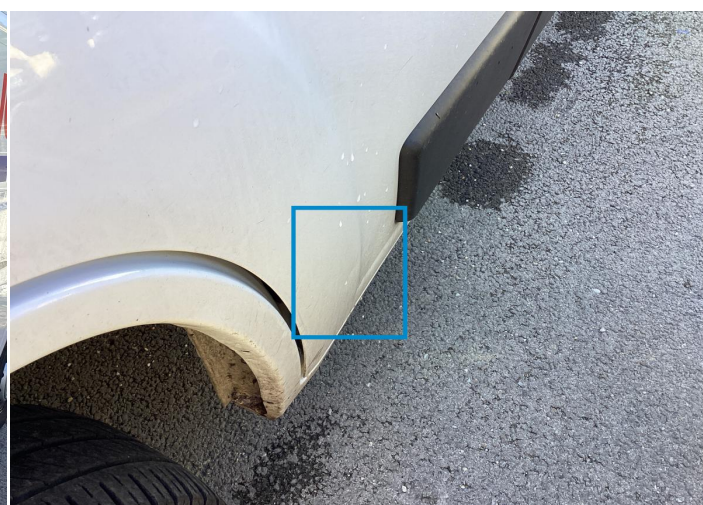
12. Door / Front Left Bodywork / Dent / Deformation -
