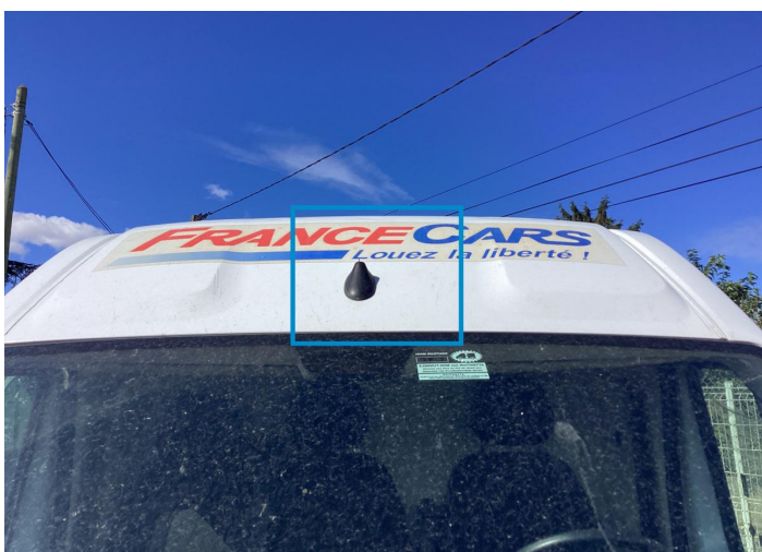
9. Antenna Rod Missing Part -
