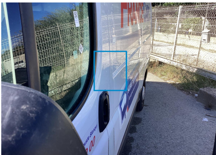
13. Door / Front Left Bodywork / Dent / Deformation -
