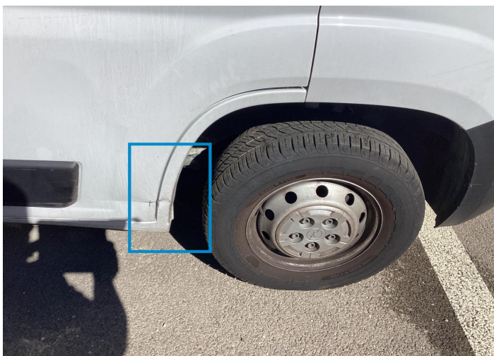
7. Fender / Front Right Bodywork / Dent / Deformation -
