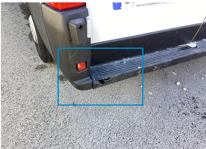
18. Shield / Back Bodywork / Breakage -
