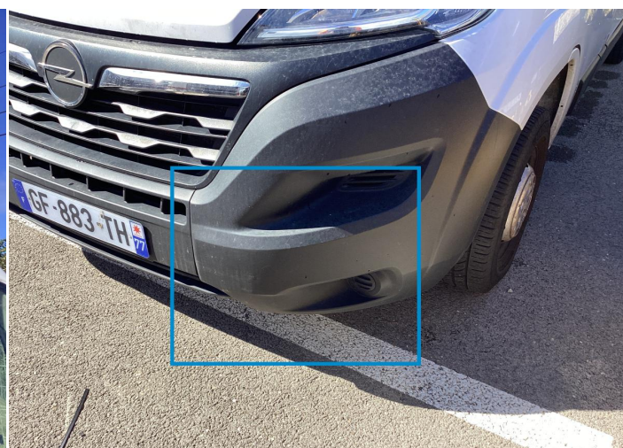
10. Shield / Front Bodywork / Dent / Deformation -
