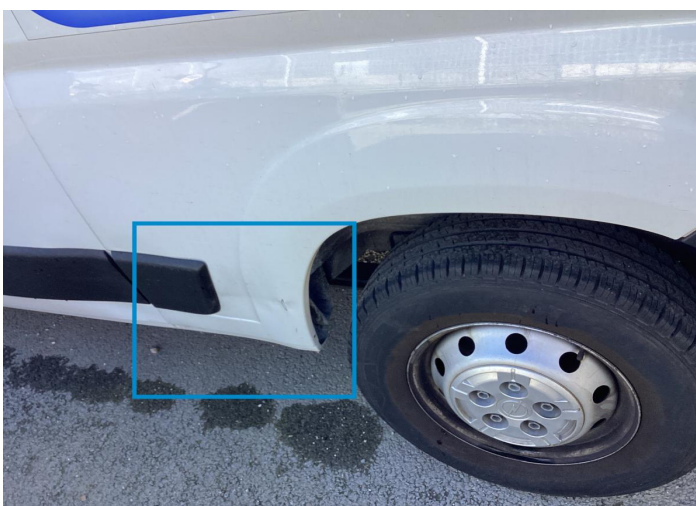
16. Fender / Back Left Bodywork / Dent / Deformation -
