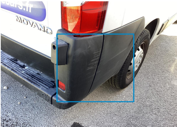
2. Shield / Back Paint / Scratch / Line -
