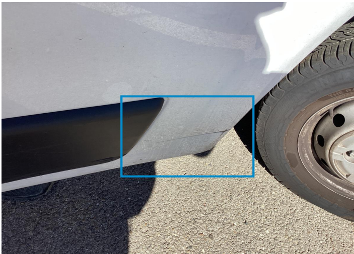
5. Door / Front Right Bodywork / Dent / Deformation -
