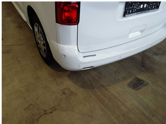
Damage 3: Rear bumper: Rear bumper - Deformed - Replace
