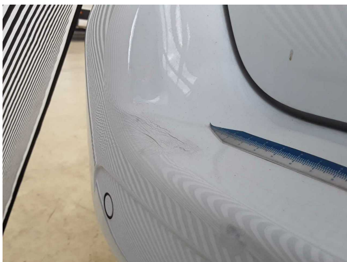
Damage 3: Rear bumper: Rear bumper - Deformed - Replace
