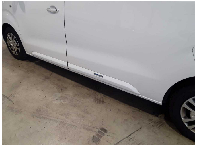
Damage 1: Side panel - rear left side: Brightware - Scratched - Paint
