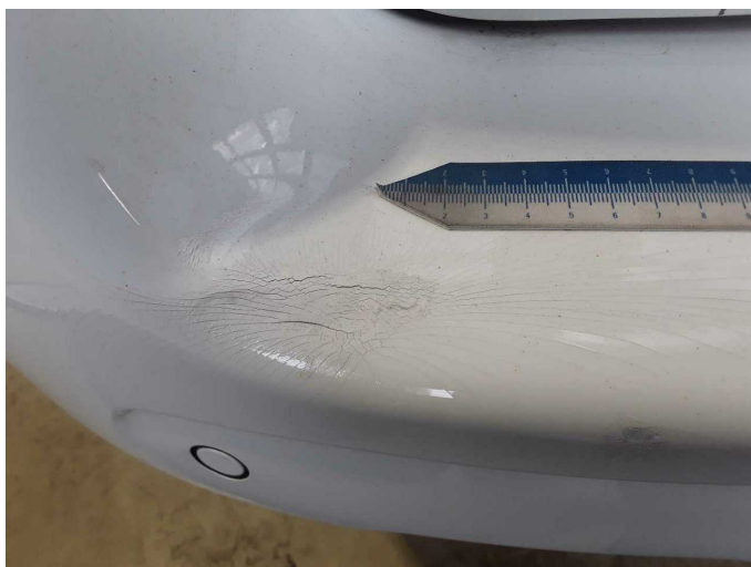
Damage 3: Rear bumper: Rear bumper - Deformed - Replace
