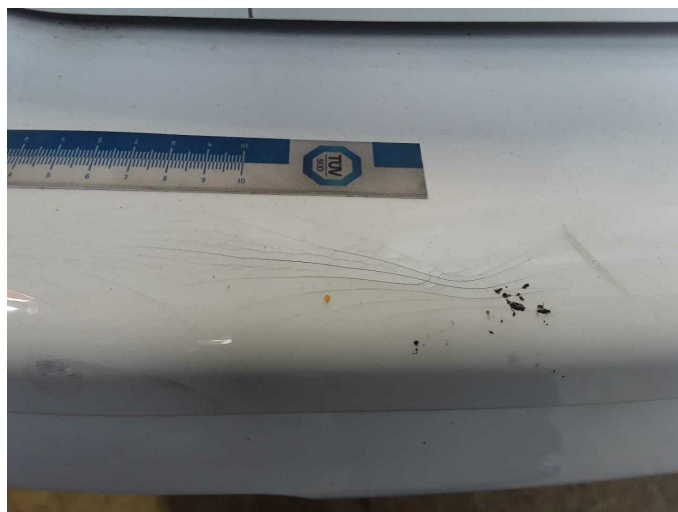
Damage 3: Rear bumper: Rear bumper - Deformed - Replace
