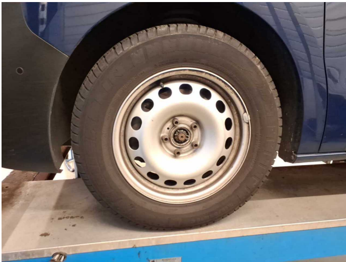
Damage 1: Wheel / tyres: Hubcap (4x) - Missing - Replace
