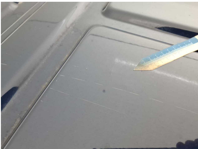
Damage 16: Roof: Roof - Dent / paintcoat damage - Repair and paint
