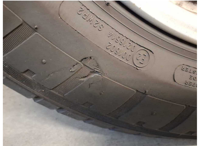
Damage 4: Wheel / tyres: Tyre - front left side - Damaged - Replace
