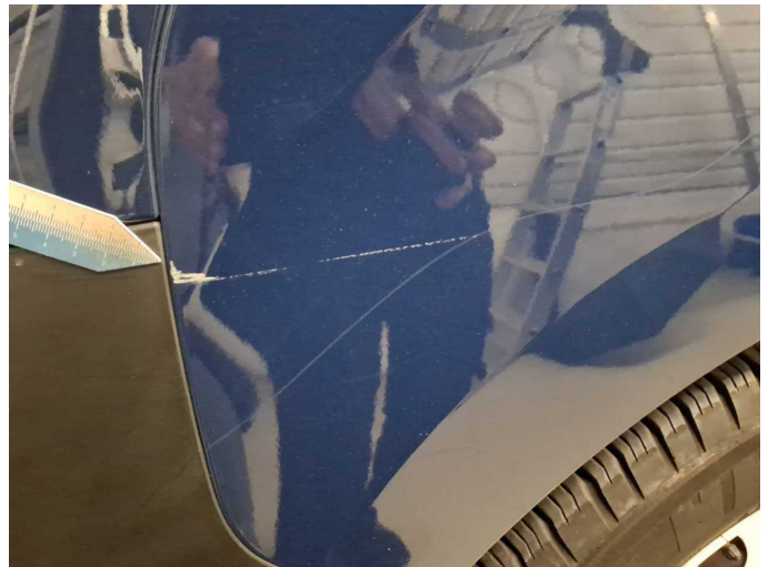
Damage 7: Mudguard - left side: Mudguard - left side - Scratch(es) - Paint
