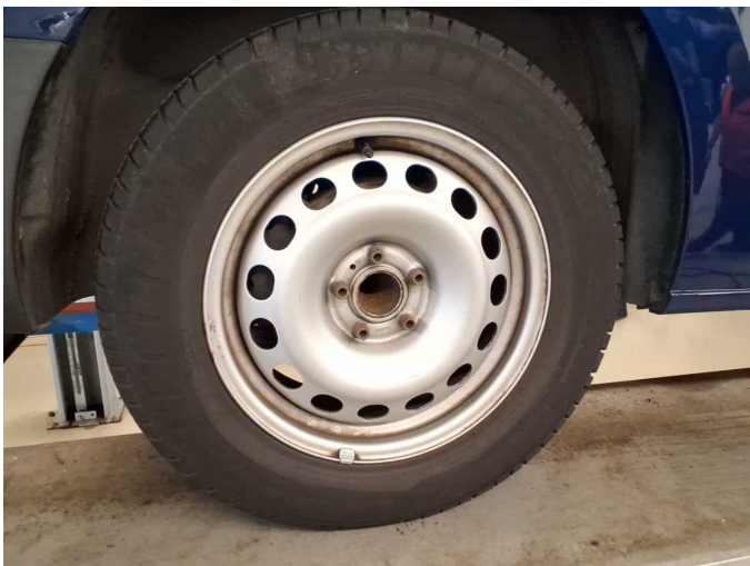
Damage 1: Wheel / tyres: Hubcap (4x) - Missing - Replace
