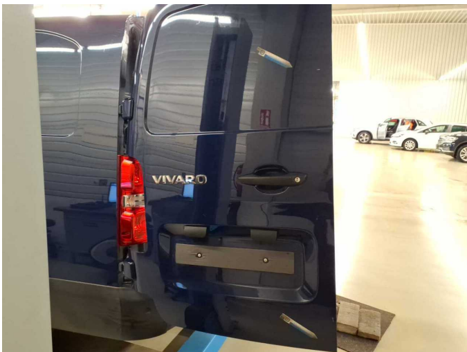
Damage 14: Boot lid / rear door: Rear door - left side - Dent / paintcoat damage - Repair and paint
