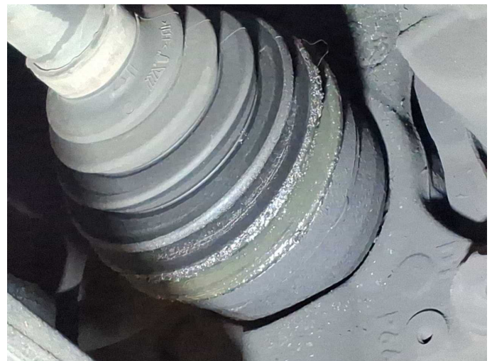
Damage 6: Drive train: Sleeve prop shaft - front left side (+ vorn rechts aussen) - Leaking - Replace
