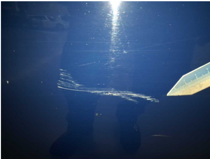
Damage 17: Sliding door, right: Sliding door - Dent / paintcoat damage - Repair and paint
