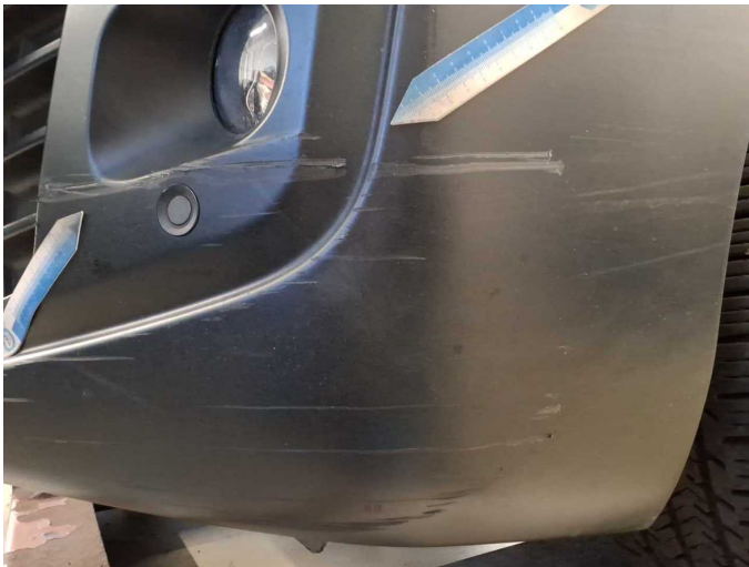
Damage 2: Front bumper: Bumper with Parktronic - Scratched - Loss in value
