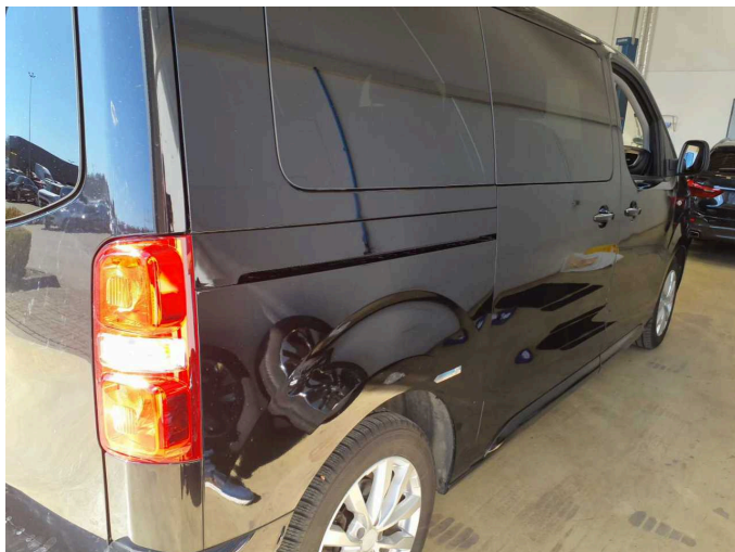
Damage 2: Side panel - rear right side: Side panel (Polieren) - Scratch(es) - Cover / polish
