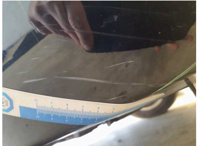
Damage 6: Front bumper: Front bumper - Paint defect - Repair and paint
