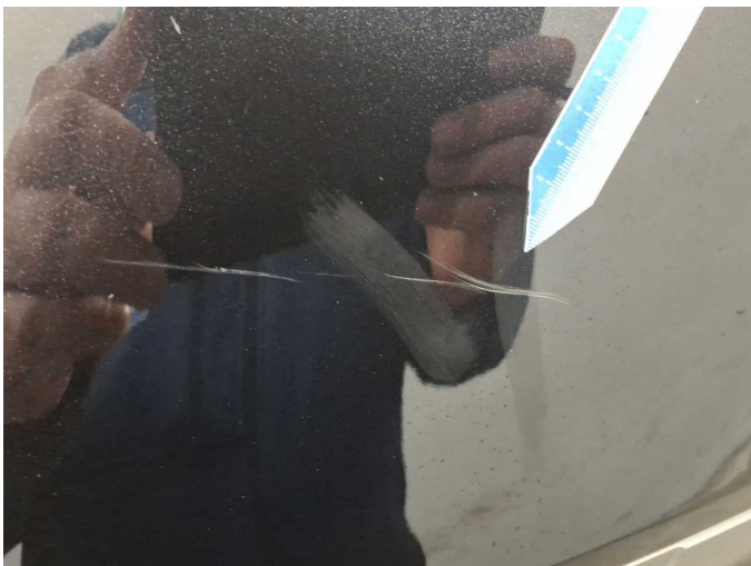
Damage 4: Rear bumper: Rear bumper - Scratched - Paint
