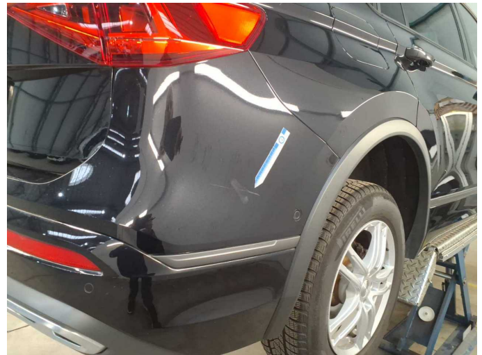
Damage 4: Rear bumper: Rear bumper - Scratched - Paint
