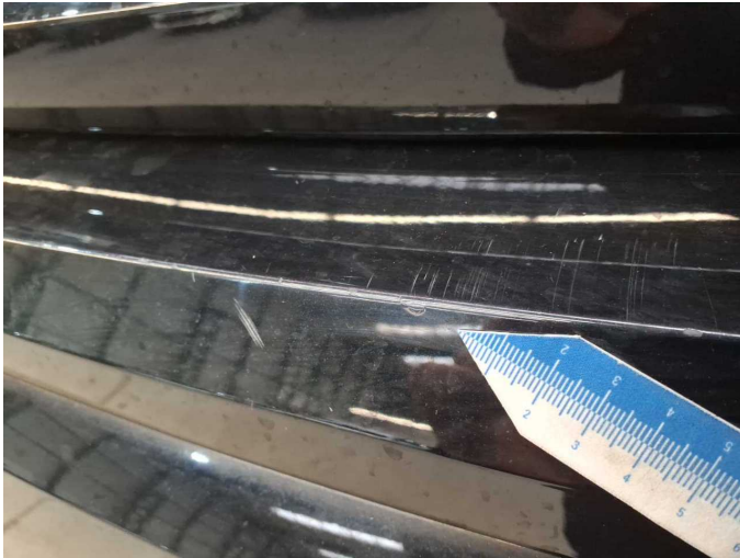
Damage 4: Rear bumper: Rear bumper - Scratched - Paint
