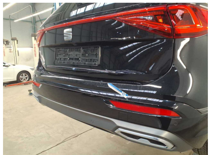
Damage 4: Rear bumper: Rear bumper - Scratched - Paint
