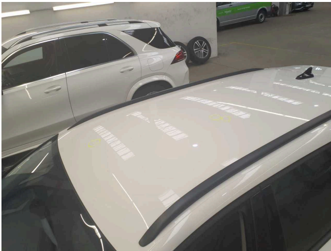
Damage 2: Roof: Roof - dent(s) - Smart repair
