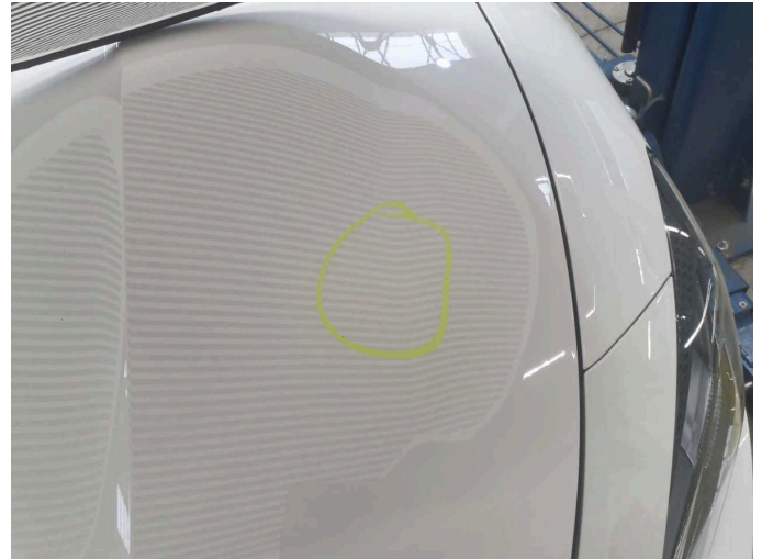
Damage 1: Bonnet: Bonnet - dent(s) - Smart repair
