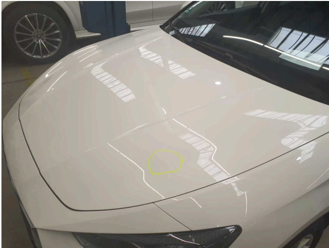
Damage 1: Bonnet: Bonnet - dent(s) - Smart repair
