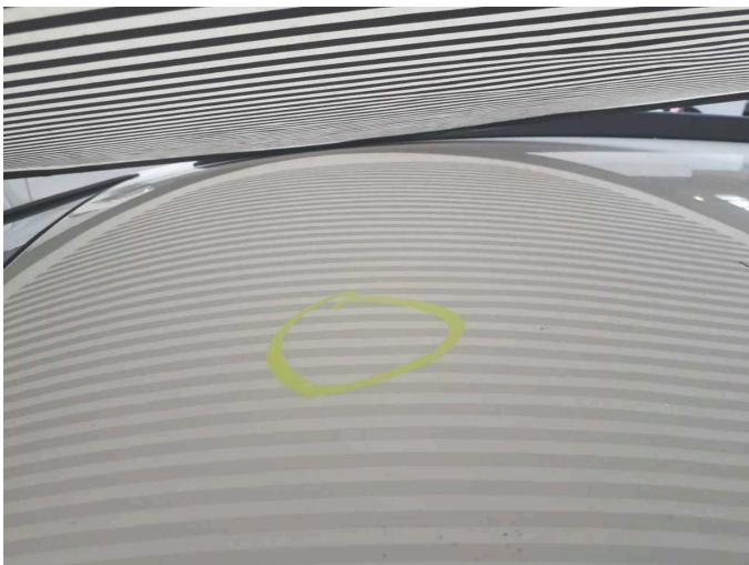
Damage 2: Roof: Roof - dent(s) - Smart repair
