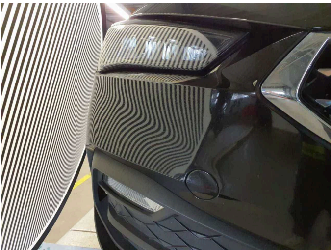
Damage 4: Front bumper: Front bumper (Steinschlag) - Scratched - Paint
