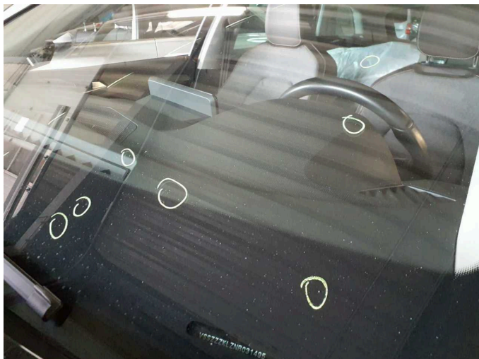
Damage 5: Vehicle glazing: Windscreen (Sandstrahleffekt) - Stone chips - Replace
