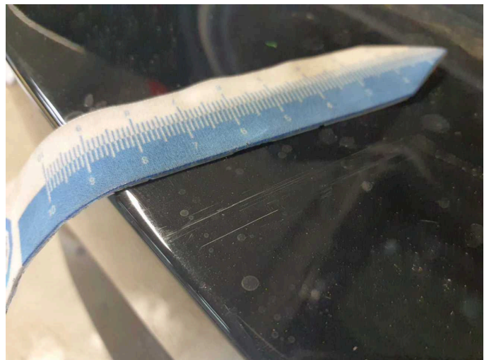
Damage 3: Rear bumper: Rear bumper - Scratched - Paint
