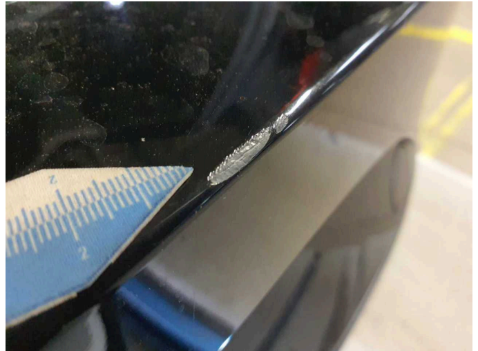
Damage 3: Rear bumper: Rear bumper - Scratched - Paint
