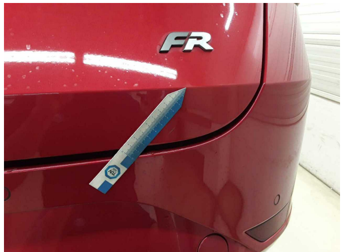
Damage 3: Boot lid / rear door: Boot lid (Unterteil) - Scratch(es) - Repair and paint
