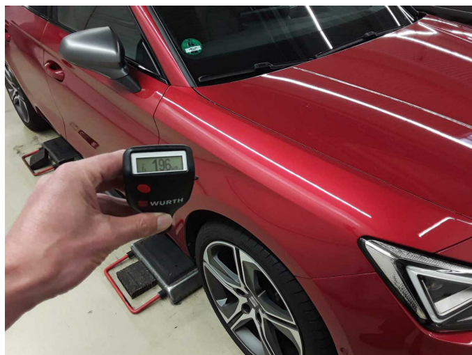
Mudguard - right side: 196 µm
