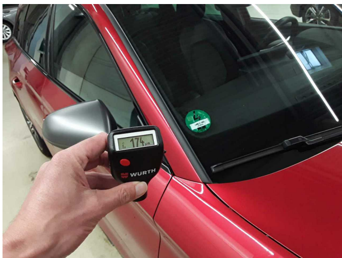
Roof rail - right side: 174 µm
