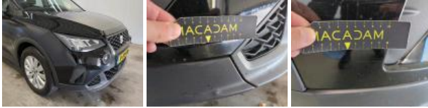
Bumper moulding FR, Dent(s) and scratch(es), Replace
