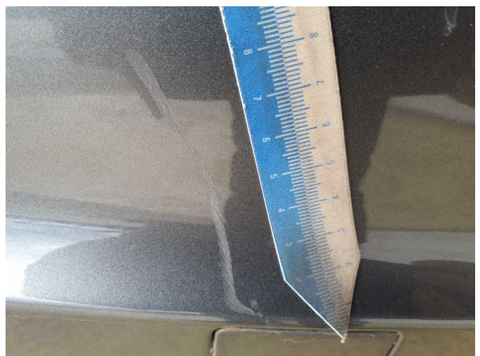
Damage 9: Rear bumper: Rear bumper - Scratch(es) - Paint
