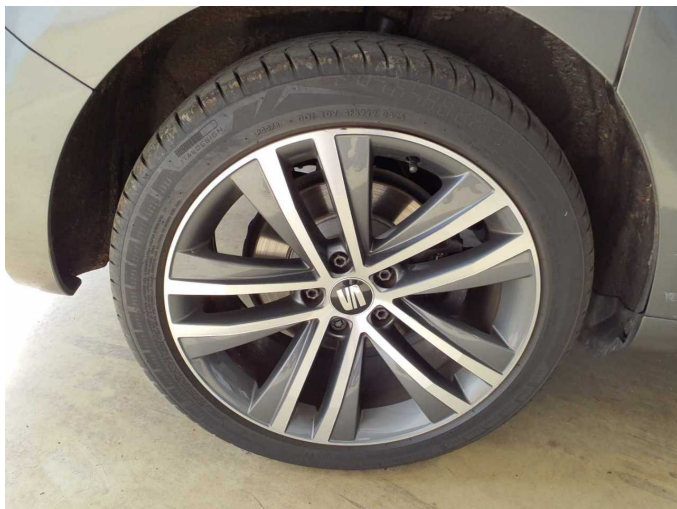
Wear and tear 7: Wheel / tyres: Alloy rim - rear right side - Scratch(es) - No deduction
