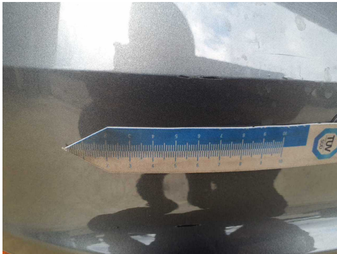
Damage 9: Rear bumper: Rear bumper - Scratch(es) - Paint
