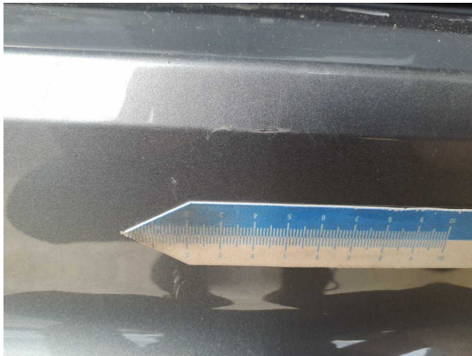
Damage 9: Rear bumper: Rear bumper - Scratch(es) - Paint
