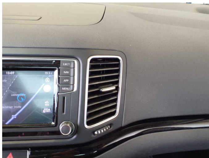
Damage 6: Instrument panel: Air nozzle - centre - Damaged - Replace
