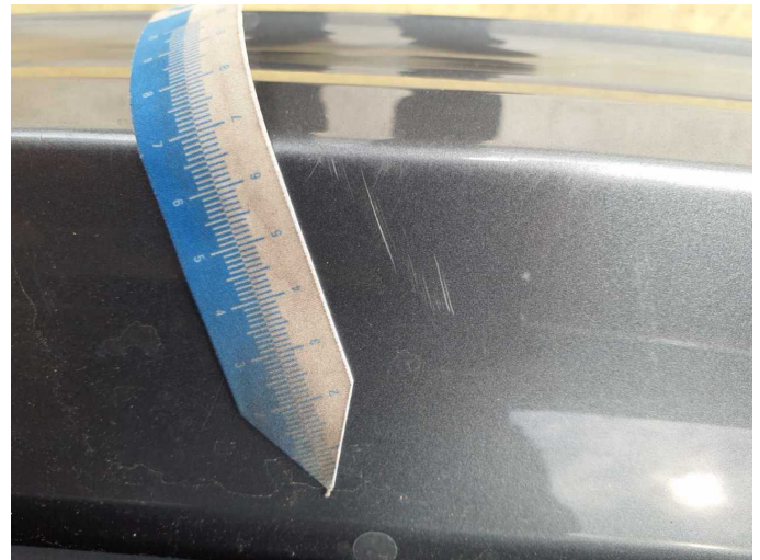
Damage 9: Rear bumper: Rear bumper - Scratch(es) - Paint
