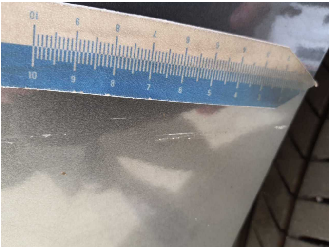
Damage 9: Rear bumper: Rear bumper - Scratch(es) - Paint
