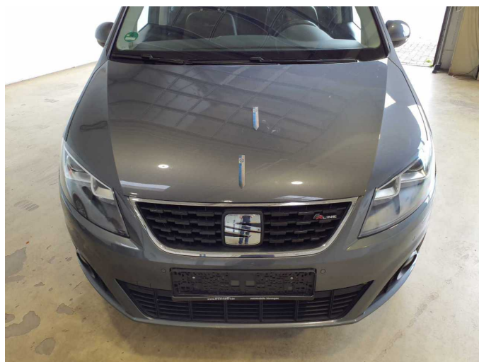
Damage 7: Bonnet: Bonnet (+ Harz) - Stone chips - Paint
