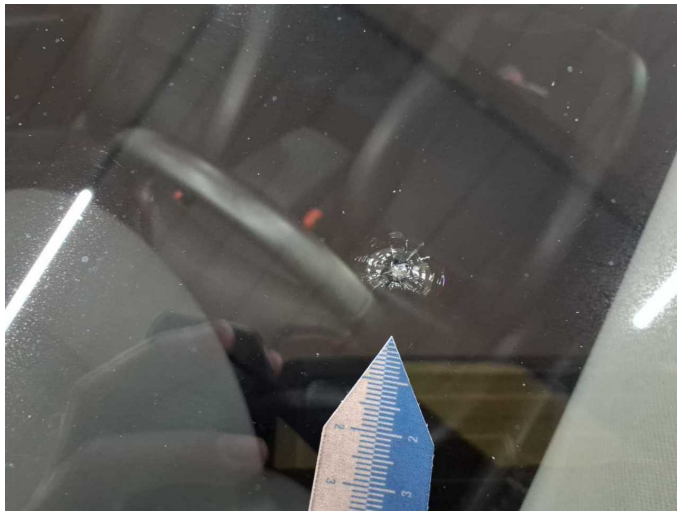
Damage 9: Vehicle glazing: Windscreen - Broken / torn - Replace
