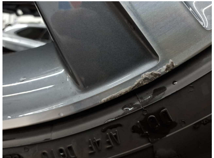
Damage 5: Wheel / tyres: Alloy rim - front right side - Scratched - Loss in value
