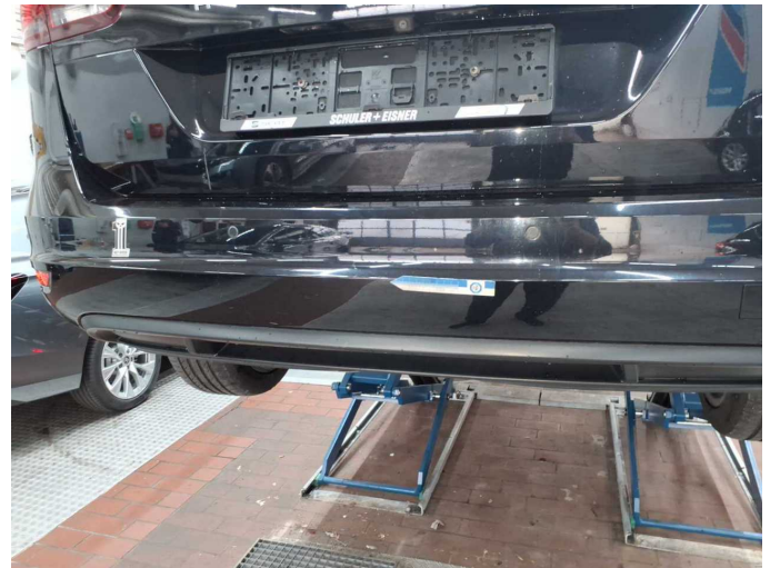
Wear and tear 1: Rear bumper: Rear bumper (Ladekante) - Scratch(es) - No deduction
