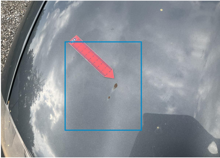
5. Hood Paint / Corrosion -
