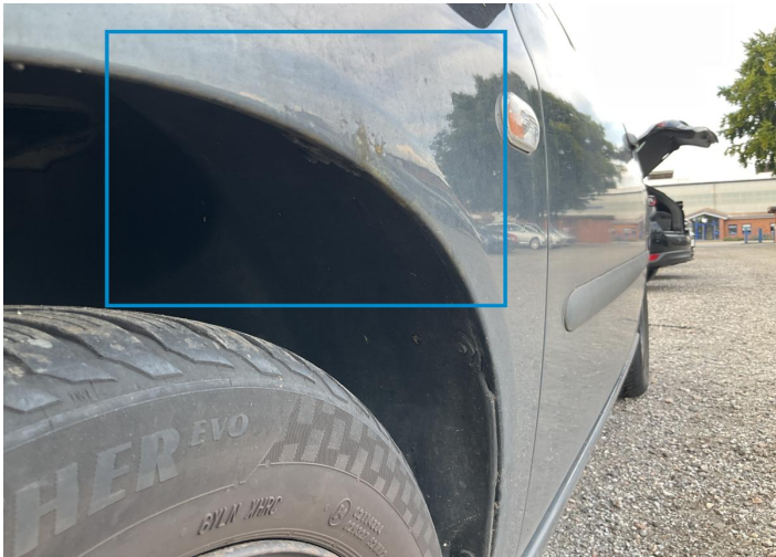
16. Fender / Front Left Paint / Corrosion -
