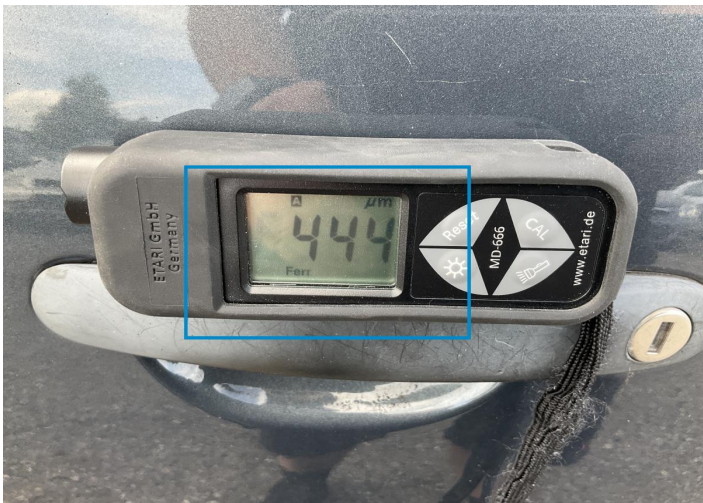
1. Door / Front Left Paint / Poor Previous Repair -
