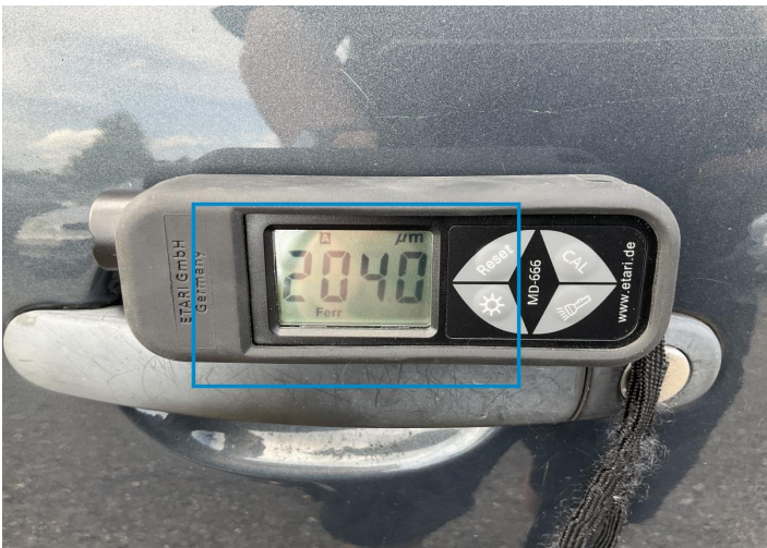
2. Fender / Back Left Paint / Poor Previous Repair -
