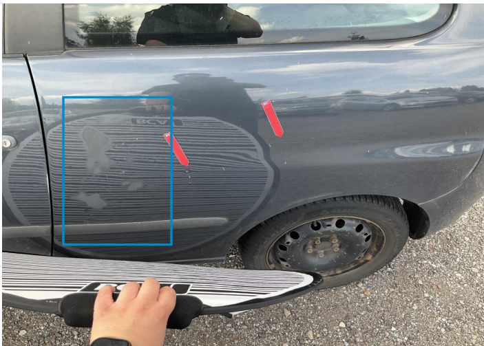
7. Fender / Back Left Paint / Poor Previous Repair -
