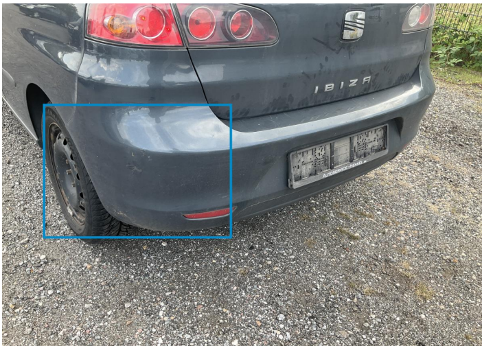
10. Bumper / Back Bodywork / Breakage / Crack -
