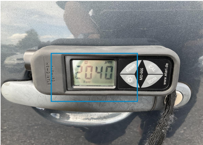
2. Fender / Back Left Paint / Poor Previous Repair -
