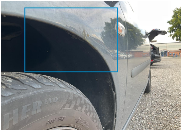
16. Fender / Front Left Paint / Corrosion -
