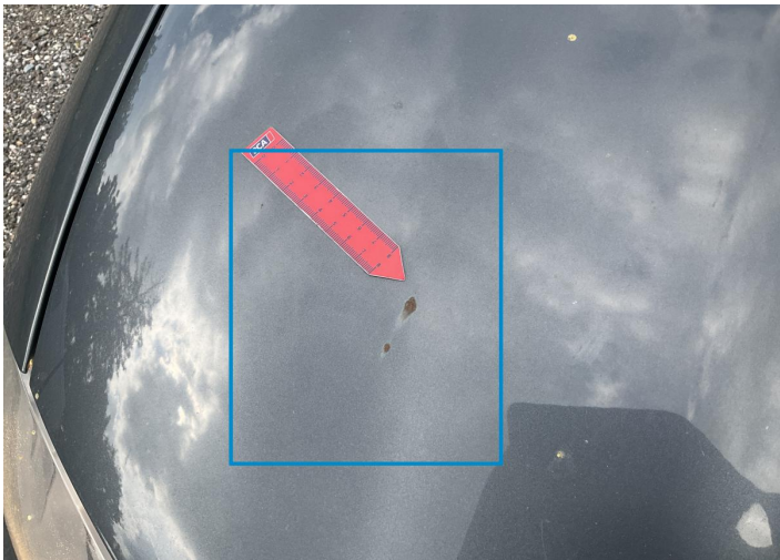
5. Hood Paint / Corrosion -
