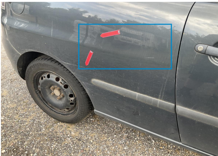
12. Fender / Back Right Paint / Scratch / Scuff -
