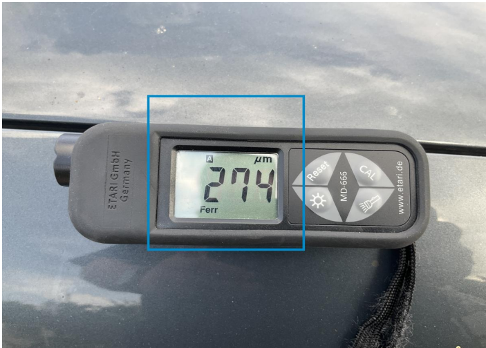
3. Fender / Front Right Paint / Poor Previous Repair -
