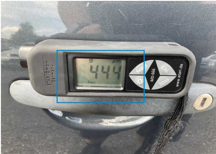
1. Door / Front Left Paint / Poor Previous Repair -
