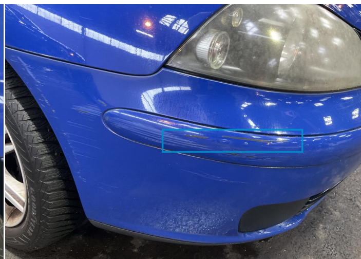
20. Corner Bumper / Front Left Paint / Corrosion -
