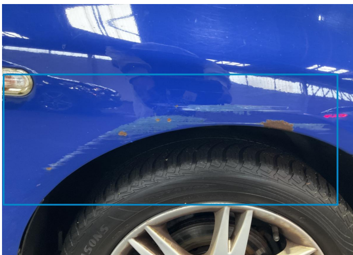
19. Fender / Front Right Paint / Scratch / Scuff -
