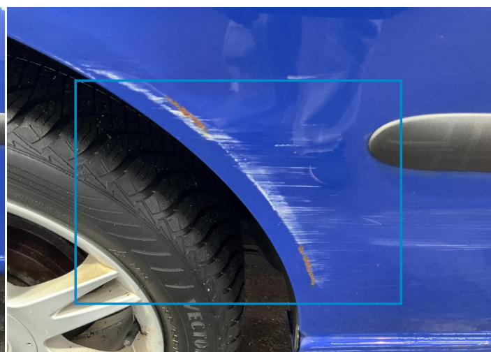
14. Side Panel / Back Right Paint / Corrosion -
