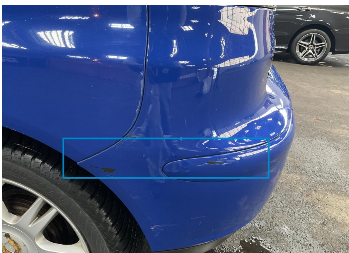
10. Bumper / Back Paint / Corrosion -
