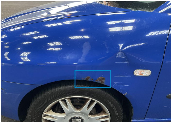
3. Fender / Front Left Paint / Corrosion -
