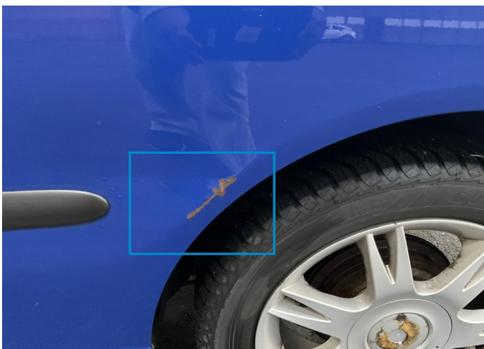
8. Side Panel / Back Left Paint / Corrosion -
