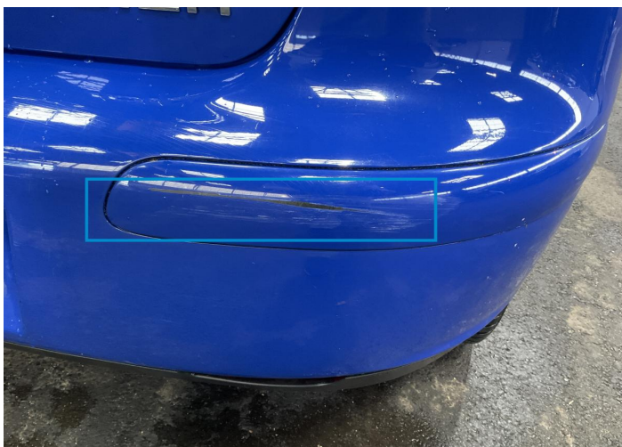
11. Corner Bumper / Back Right Paint / Scratch / Scuff -
