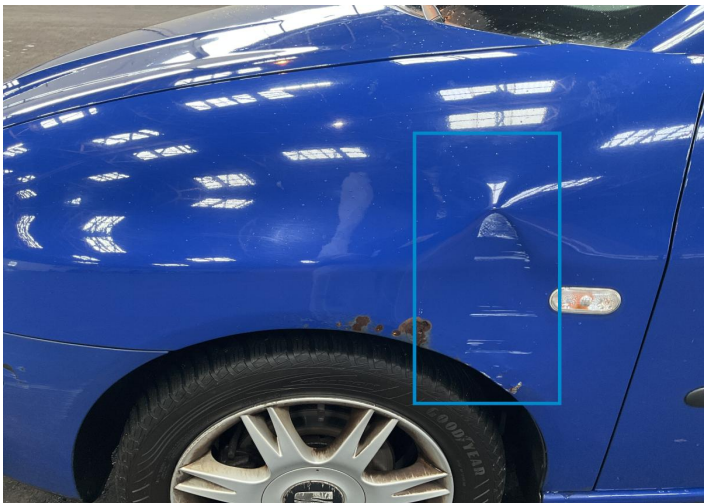
2. Fender / Front Left Bodywork / Dent / Dent -
