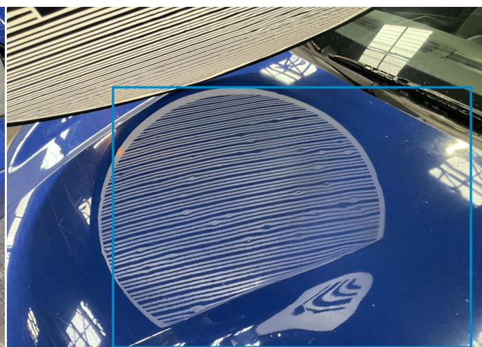
22. Hood Bodywork / Dent / Hail Area -
