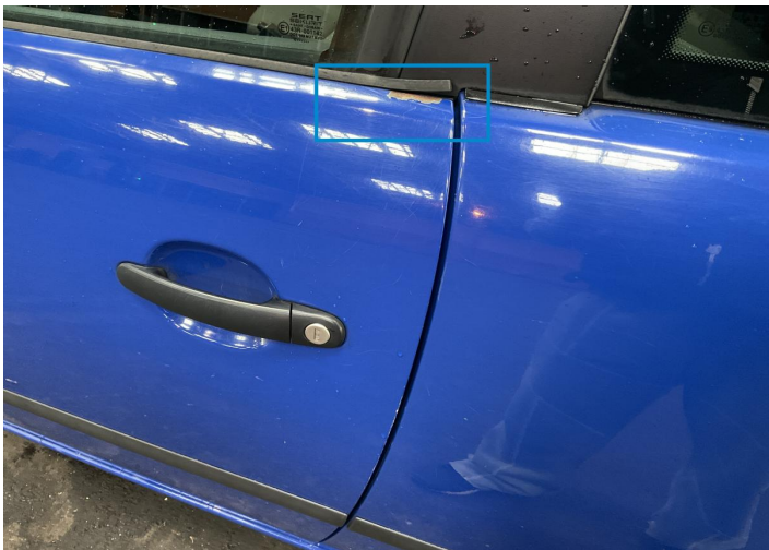
4. Door / Front Left Paint / Corrosion -
