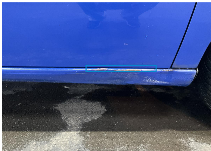
17. Rocker Panel / Center Right Paint / Corrosion -
