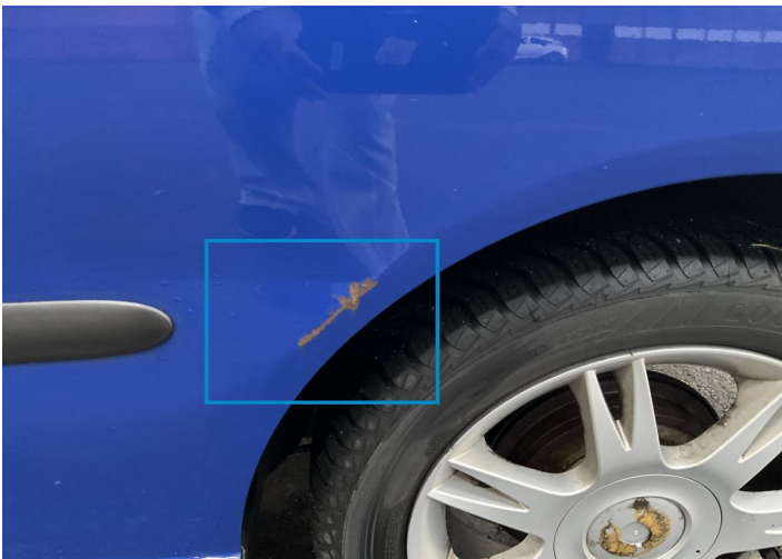
8. Side Panel / Back Left Paint / Corrosion -
