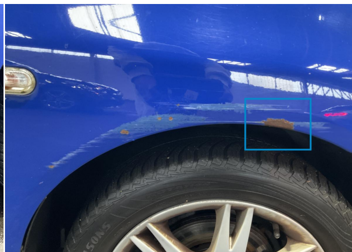
18. Fender / Front Right Paint / Corrosion -
