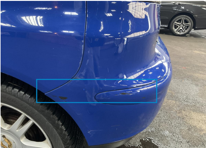
10. Bumper / Back Paint / Corrosion -
