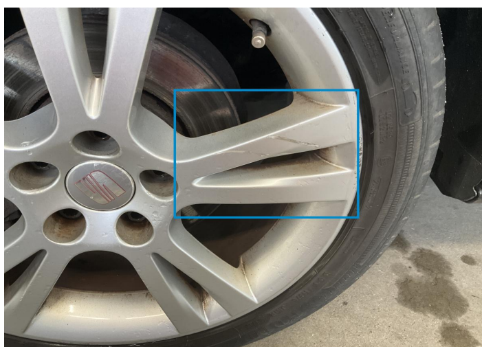
5. Rim / Front Left Out of Bodywork / Scratch -
