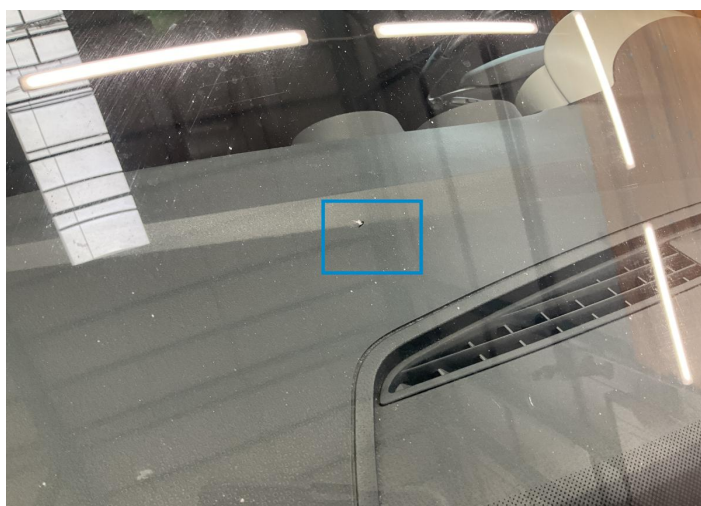
3. Windshield / Front Paint / Chipping -
