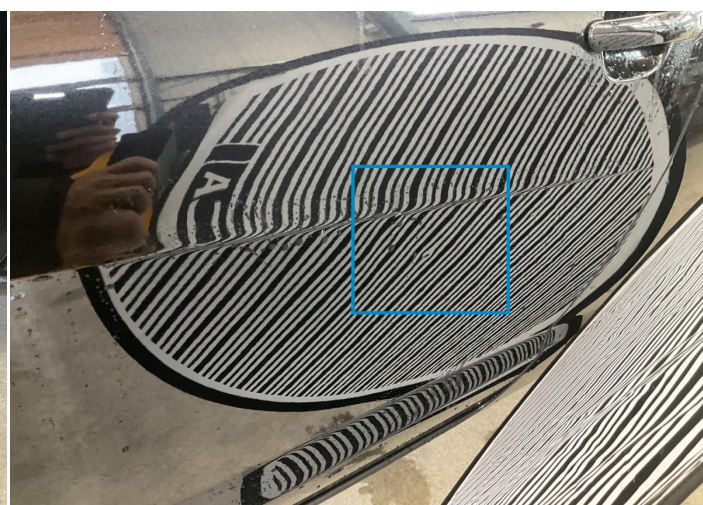
6. Door / Front Left Bodywork / Dent / Dent -
