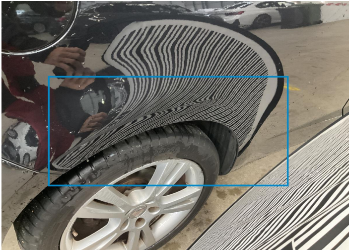
17. Fender / Back Right Bodywork / Dent / Dent -
