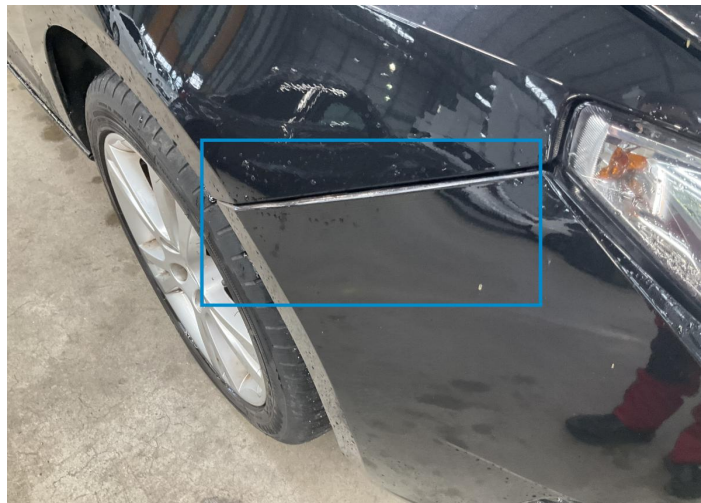
25. Bumper / Front Bodywork / Dent / Dent -
