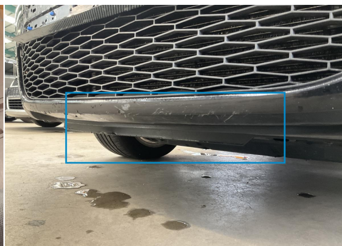
4. Bumper / Front Paint / Scratch / Scuff -
