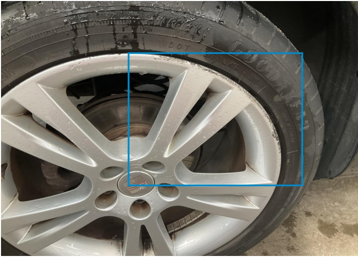
18. Rim / Back Right Out of Bodywork / Scratch -
