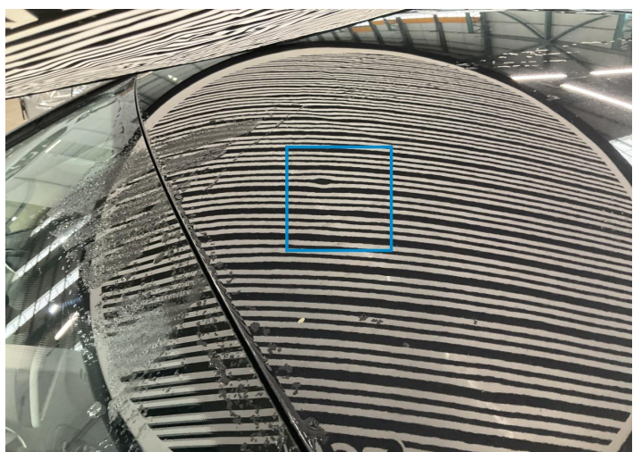
7. Roof Bodywork / Dent / Dent -
