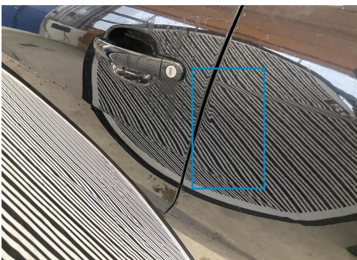
10. Fender / Back Left Bodywork / Dent / Dent -
