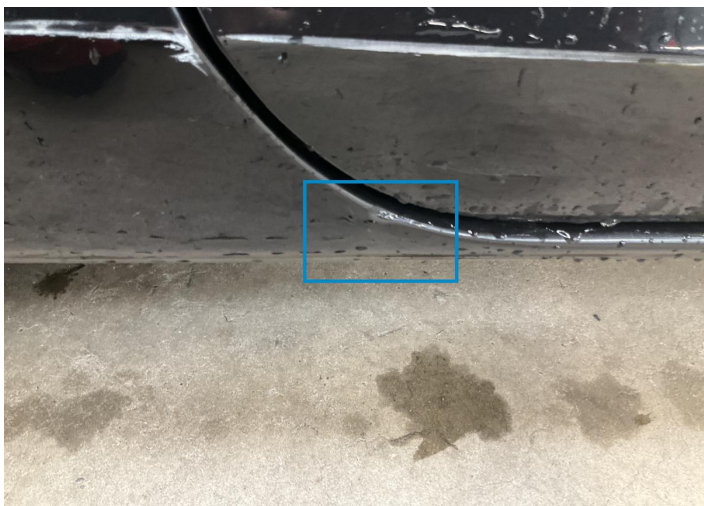
21. Rocker Panel / Center Right Bodywork / Dent / Dent -
