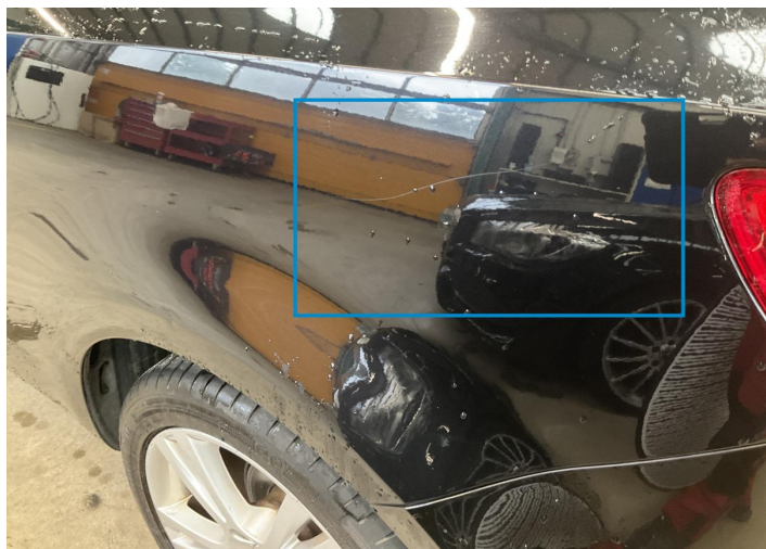
9. Fender / Back Left Paint / Scratch / Scuff -
