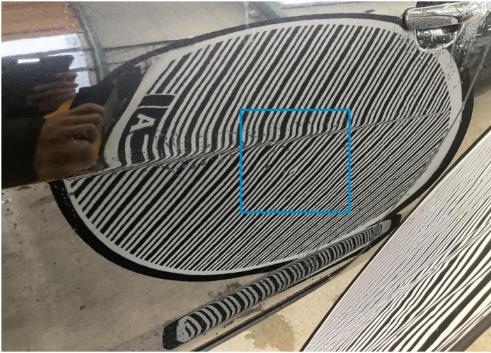
6. Door / Front Left Bodywork / Dent / Dent -
