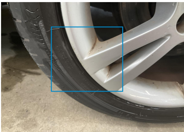
23. Rim / Front Right Out of Bodywork / Scratch -
