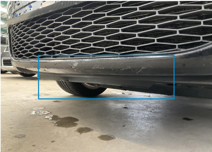
4. Bumper / Front Paint / Scratch / Scuff -
