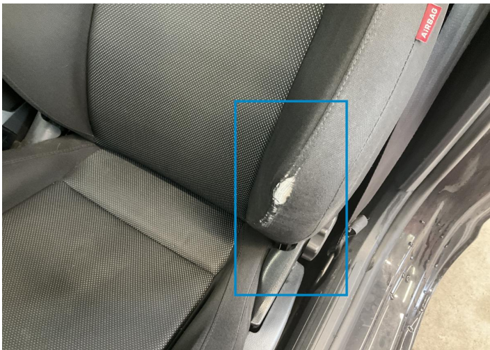
8. Seat / Front Left Interior / Ripped -
