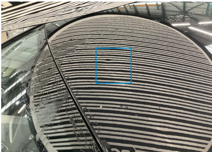
7. Roof Bodywork / Dent / Dent -
