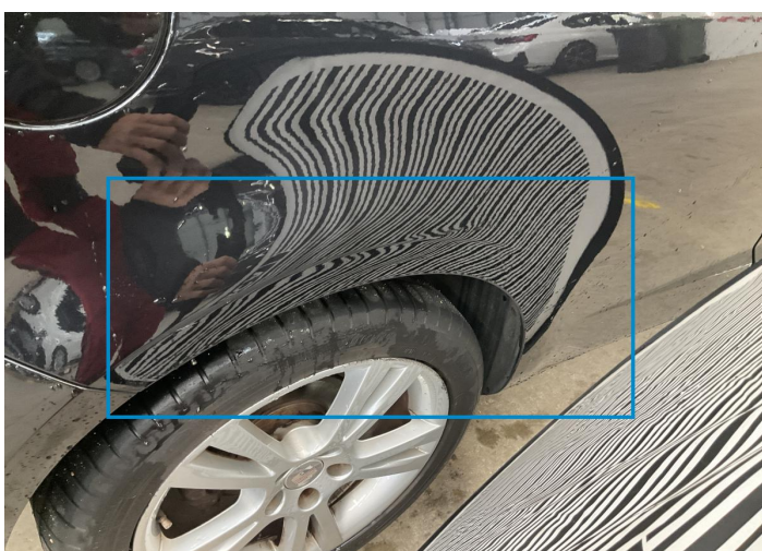
17. Fender / Back Right Bodywork / Dent / Dent -
