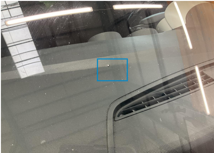
3. Windshield / Front Paint / Chipping -
