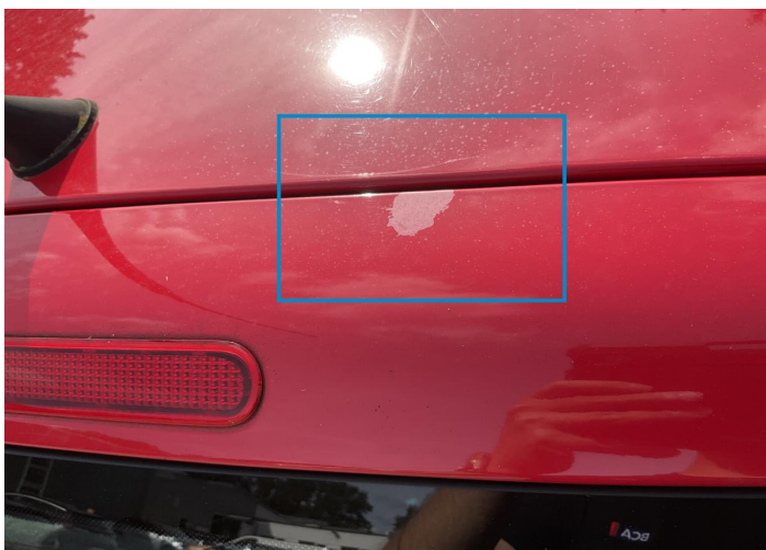
17. Tailgate Paint / Chipping -
