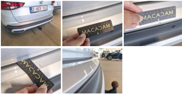
Bumper moulding R, Dent(s), Replace
