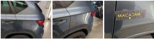
Door trim FL, Scratch(es), Replace and paint
