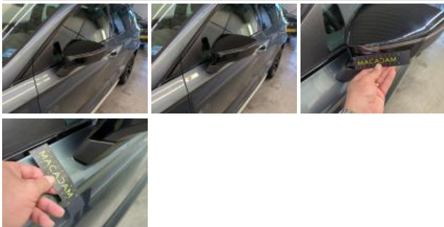
Door FR, Scratch(es), Repair and paint (complete)
