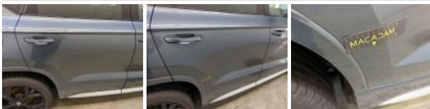
Door trim RR, Scratch(es), Replace and paint
