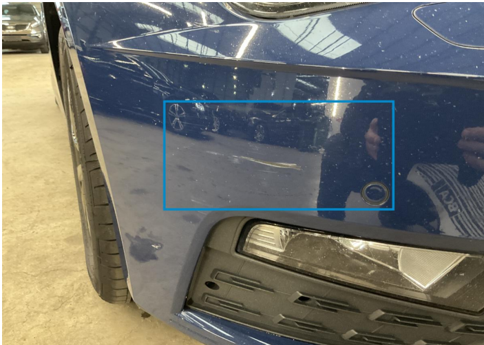
1. Bumper / Front Paint / Scratch / Scuff -
