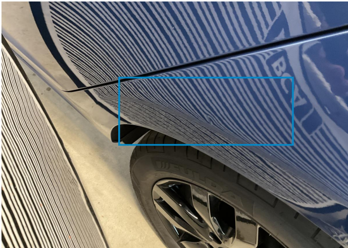
3. Fender / Back Left Bodywork / Dent / Dent -
