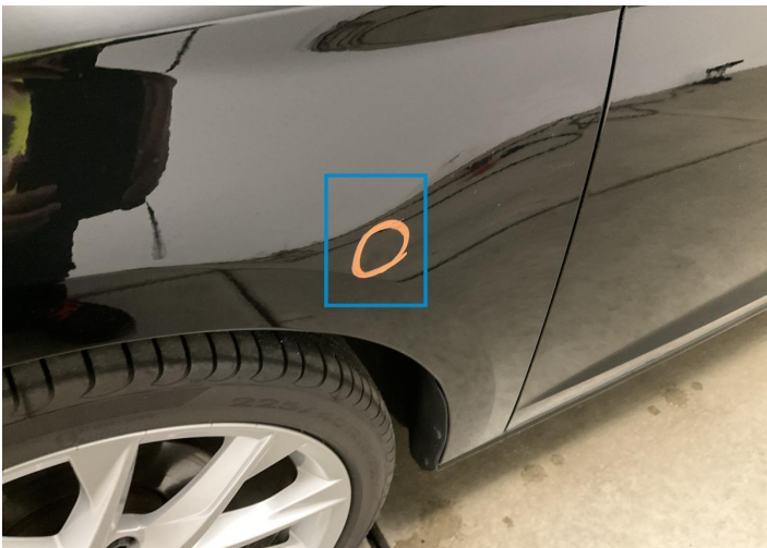
2. Fender / Front Left Bodywork / Dent / Dent -
