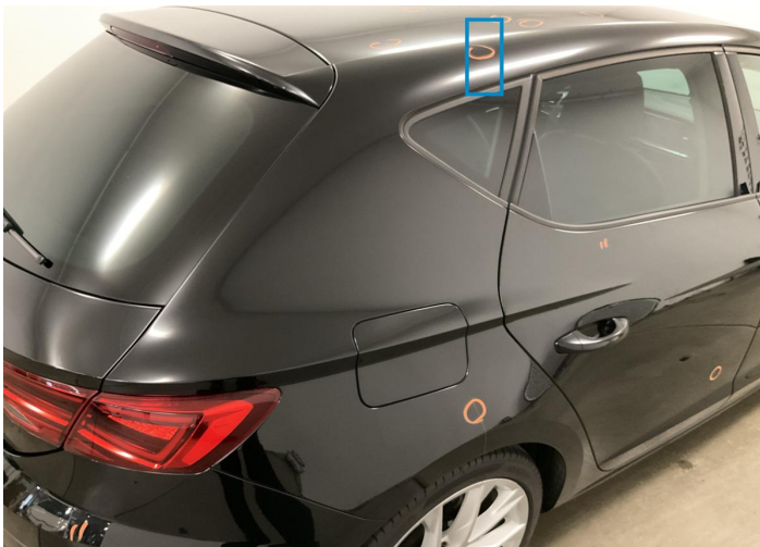
7. Side Panel / Back Right Bodywork / Dent / Dent -
