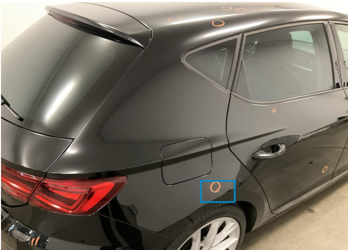
6. Side Panel / Back Right Bodywork / Dent / Dent -
