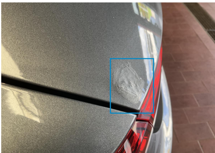
5. Tailgate Paint / Poor Previous Repair -
