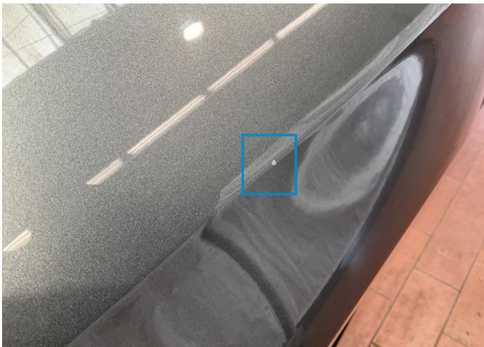
10. Fender / Front Left Paint / Stone Chip -
