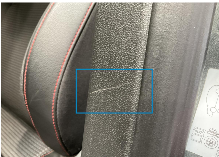
2. Panel Filling / Front Left Interior / Scratched -
