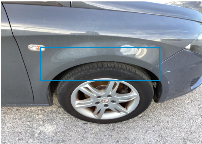
8. Fender / Front Right Bodywork / Dent / Deformation -
