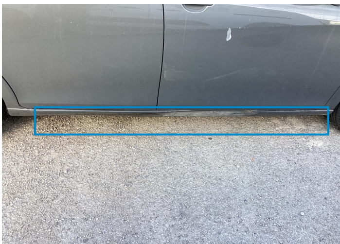
13. Rocker Panel / Center Right Bodywork / Dent / Deformation -
