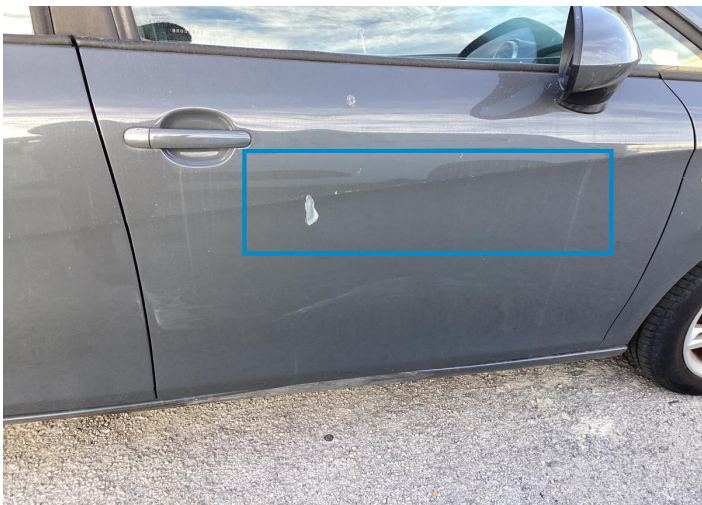
12. Door / Front Right Bodywork / Dent / Deformation -
