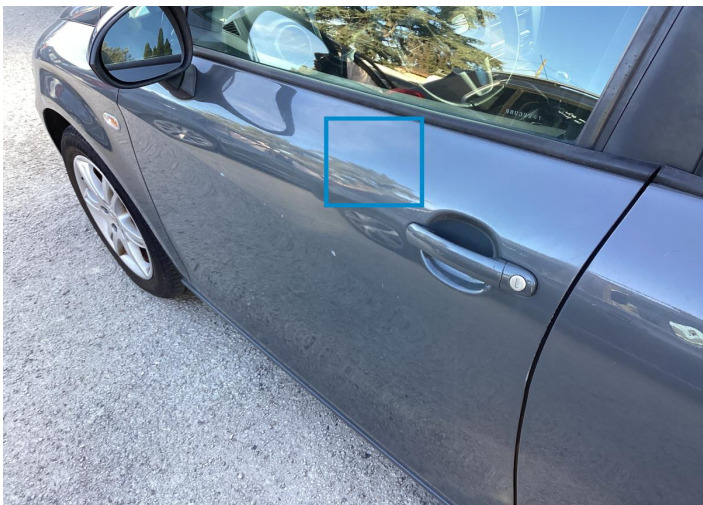
23. Door / Front Left Bodywork / Dent / Deformation -
