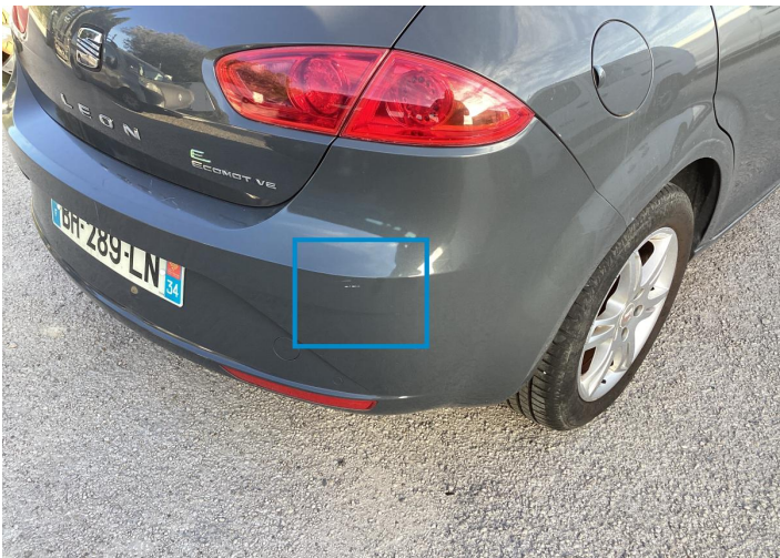
20. Shield / Back Paint / Scratch / Line -
