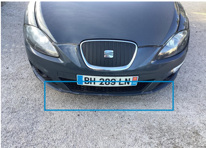
10. Shield / Front Bodywork / Dent / Deformation -
