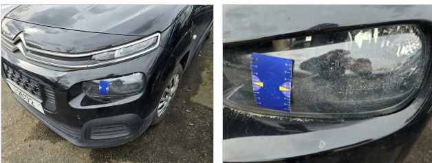
Headlight / Front left / Replace: D - Broken
