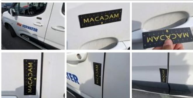
Step L, Scratch(es), Repair and paint (complete)
