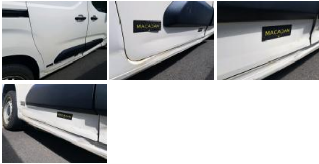
Outer sill R, Deformed / Strained, Replace and paint
