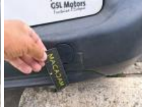
Bumper R, Broken, Replace
