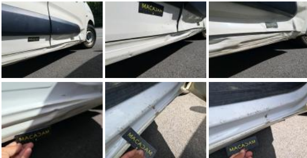
Door FR, Deformed / Strained, Replace and paint
