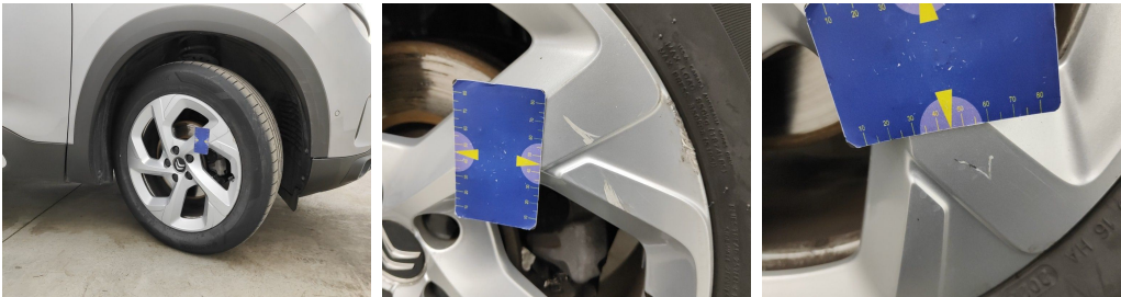
Wheel Alloy Front Right // Repair-scratch
