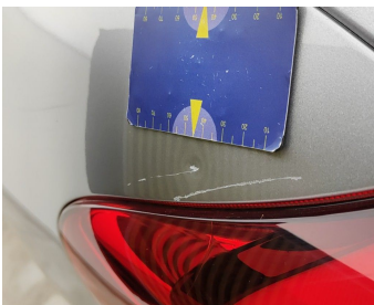
Wing Rear Left // Repair & Painting-scratch + dent
