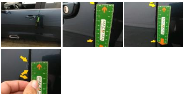
Porte ARG, Griffe(s), Acceptable
