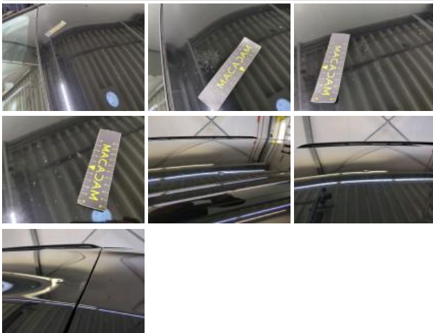
Roof, Chemical polution, Repair and paint (complete)
