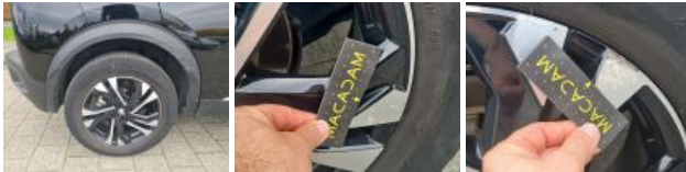
Tyre RR, Tear, Replace
