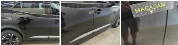
Wing RR, Dent(s), Repair and paint (complete)
