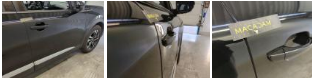
Bumper moulding R, Scratch(es), Replace and paint
