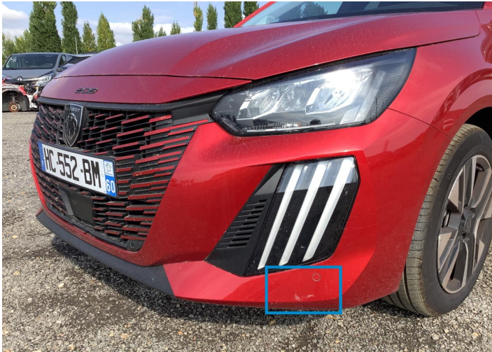
5. Corner Bumper / Front Left Paint / Scratch / Line -
