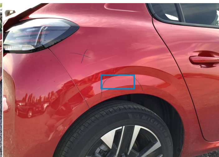
16. Fender / Back Right Bodywork / Dent / Deformation -
