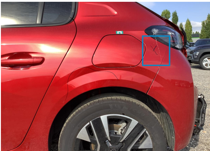
12. Fender / Back Left Paint / Scratch / Line -
