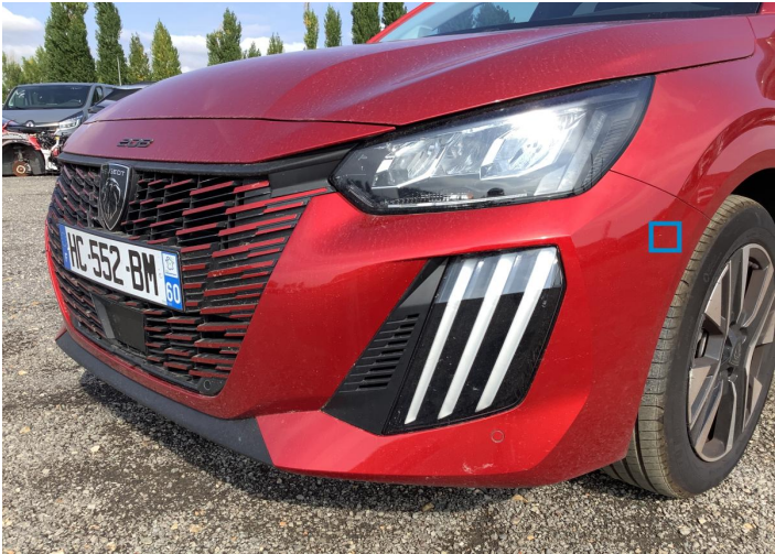
6. Corner Bumper / Front Left Paint / Scratch / Line -
