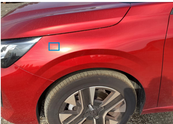
8. Fender / Front Left Paint / Scratch / Line -
