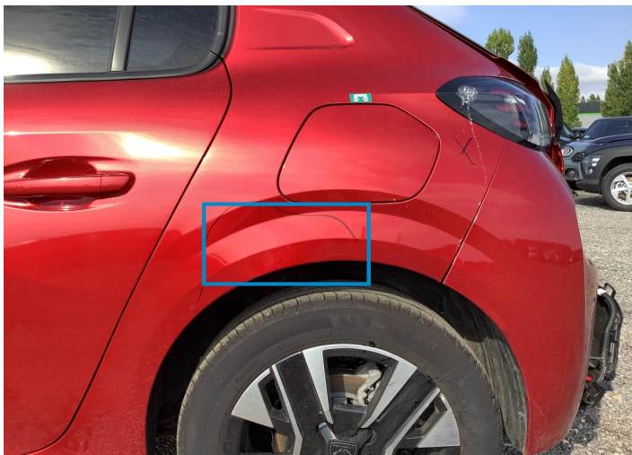
11. Fender / Back Left Bodywork / Dent / Deformation -
