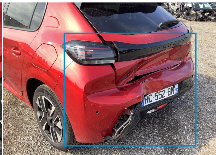
14. Corner Bumper / Back Left Bodywork / Dent / Deformation -
