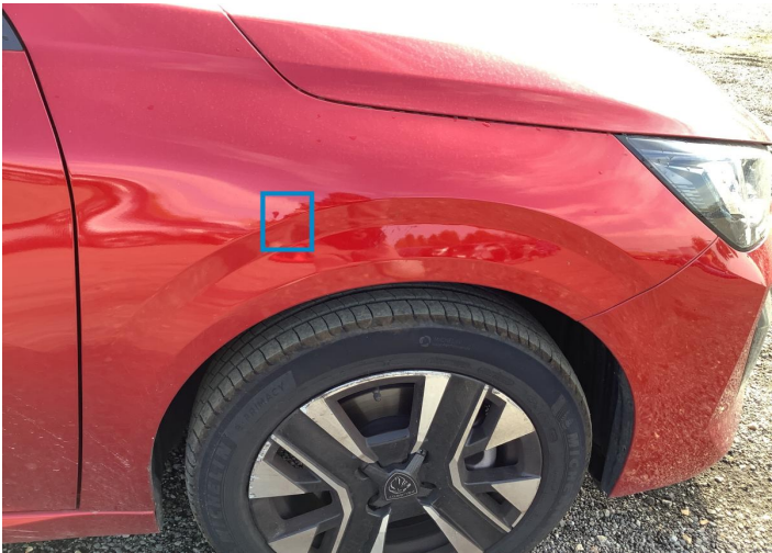
22. Fender / Front Right Bodywork / Dent / Deformation -
