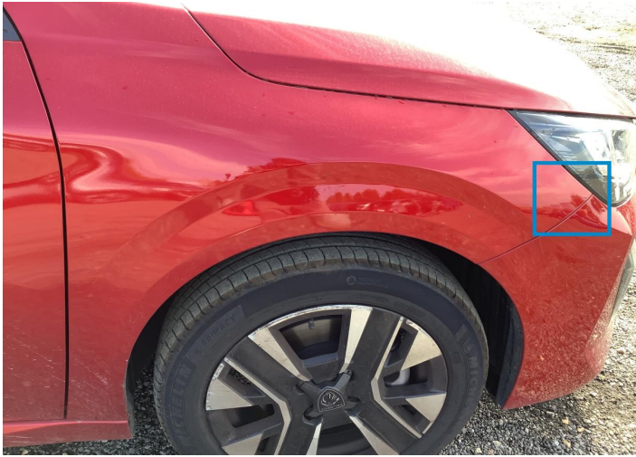
23. Fender / Front Right Paint / Scratch / Line -
