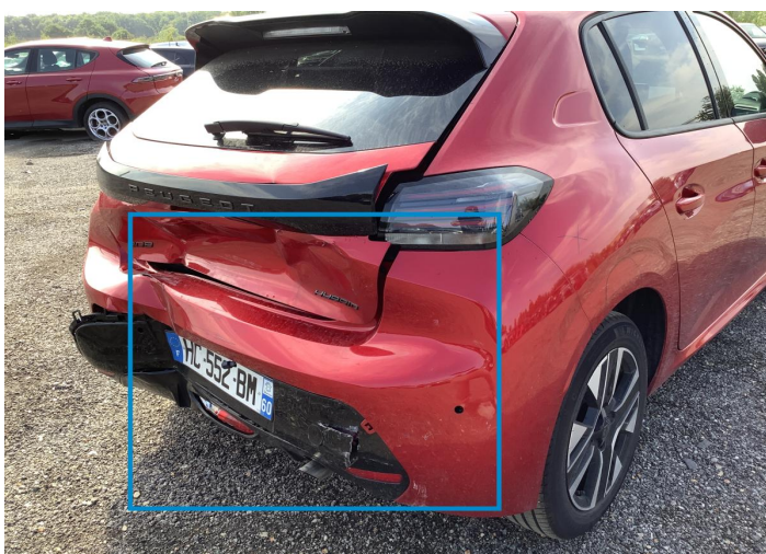
15. Corner Bumper / Back Right Bodywork / Dent / Deformation -
