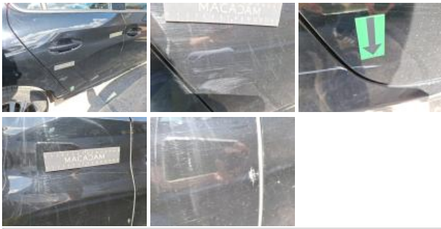
Door FR, Scratch(es), Repair and paint (complete)
