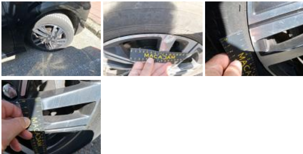
Alloy rim RR polished, Scratch(es), Repair and paint (complete)
