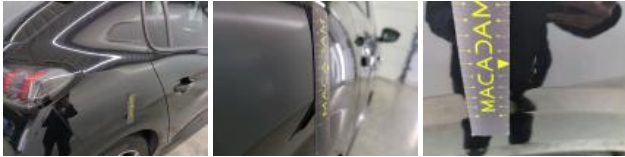
Door RR, Scratch(es), Repair and paint (complete)
