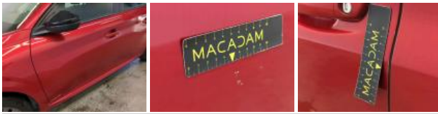
Wing FL, Scratch(es), Repair and paint (complete)
