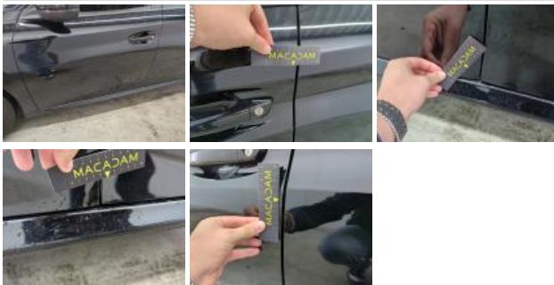
Door RL, Scratch(es), Repair and paint (partial)
