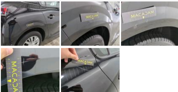
Door frame FR, Scratch(es), Repair and paint (partial)
