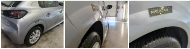
Door RR, Scratch(es), Repair and paint (complete)
