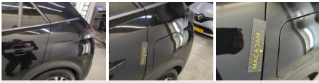
Door FR, Scratch(es), Repair and paint (complete)
