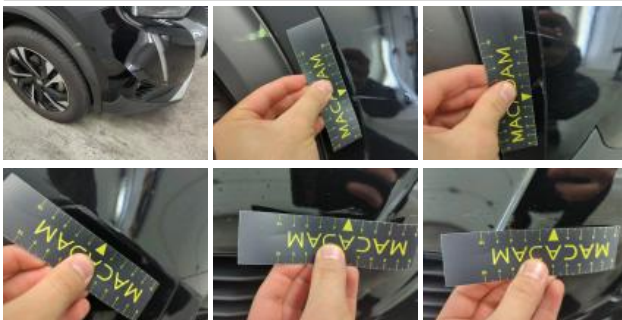
Bonnet, Scratch(es), Repair and paint (complete)
