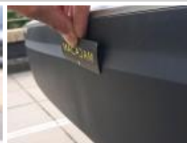
Bumper moulding R, Scratch(es), Replace
