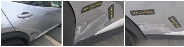
Wing trim RR, Deformed / Strained, Replace
