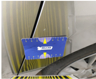
Wing Rear Left // Repair & Painting-scratch + dent
