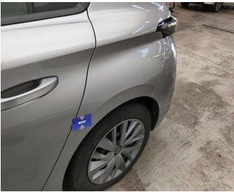
Wing Rear Left // Repair & Painting-scratch + dent
