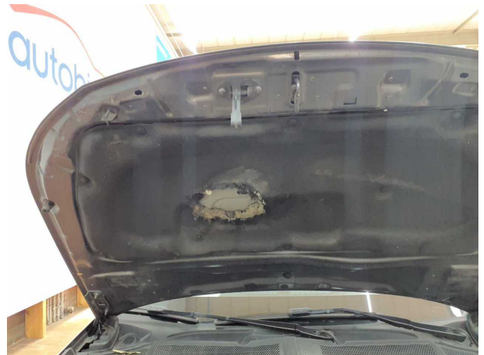
Damage 1: Bonnet: Insulation lining - Damaged - Replace
