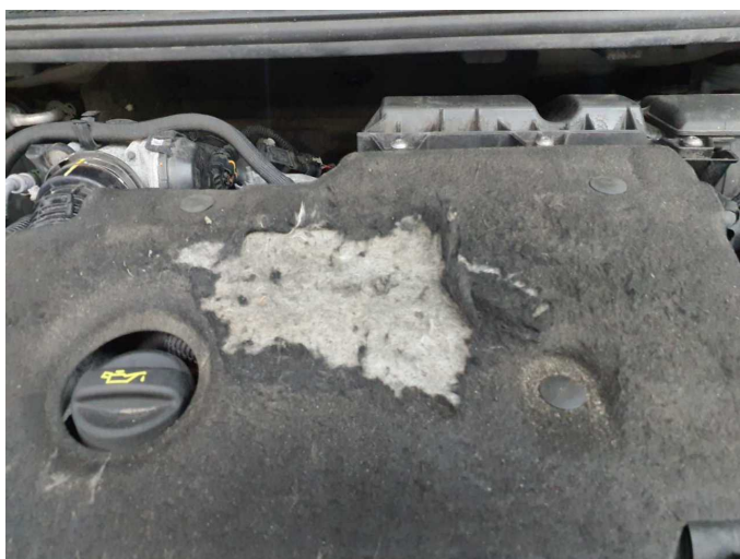
Damage 3: Engine: Engine cover - Damaged - Replace
