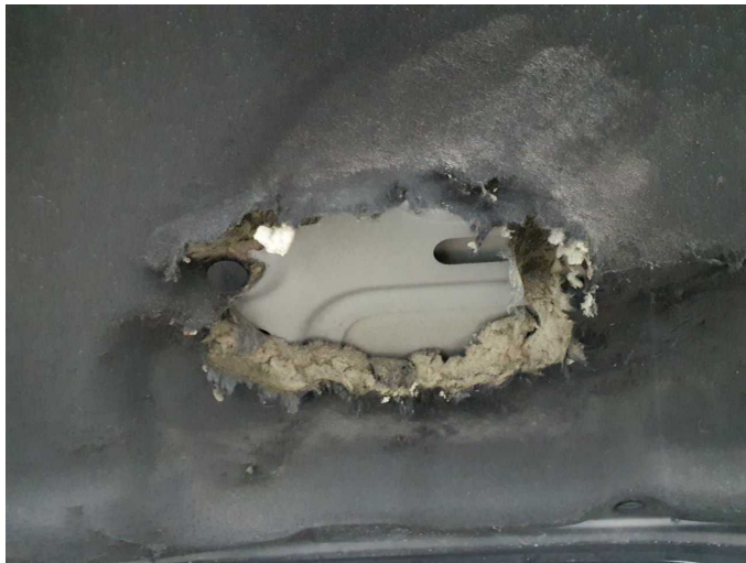
Damage 1: Bonnet: Insulation lining - Damaged - Replace
