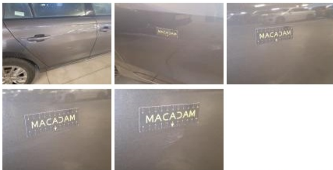
Door FR, Dent(s), Repair and paint (complete)
