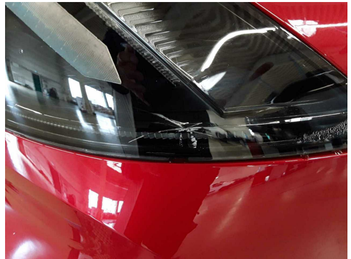
Damage 2: Tail light: Tail lamp - right side - Broken / torn - Replace
