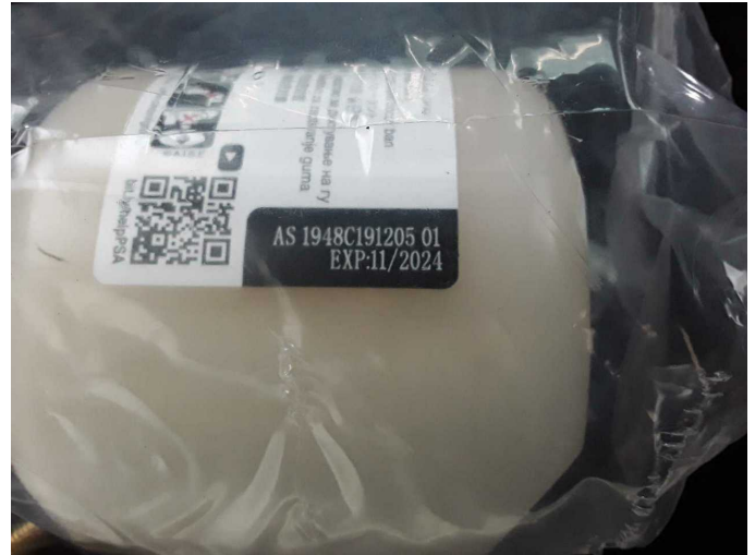
Damage 1: Equipment: Tirefit filler - Expired - Replace
